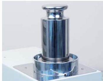
Ring-shaped draft shield encircling the weighing pan, apart from protecting the pan against air drafts, prevents potential shocks that could be applied accidentally to the weighing pan while loading the weight.
