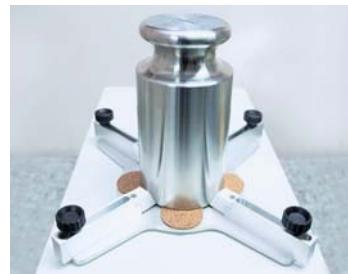
Weighing pan with mechanical centering system facilitates precise placing of mass standards, plus it reduces effect of eccentricity to zero.
