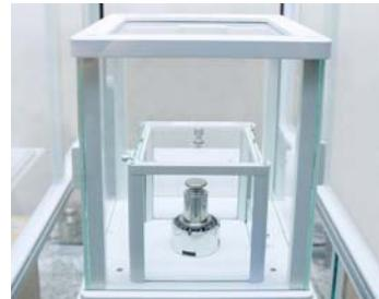
Glass draft shield minimizes influence of air drafts on comparison process. The glass with special conductive coating supports discharge of static electricity.
