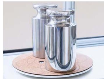
Optional “floating” self-centering pan offers reduction of eccentricity effect, plus it supports dissemination of reference mass to more than one weight.
